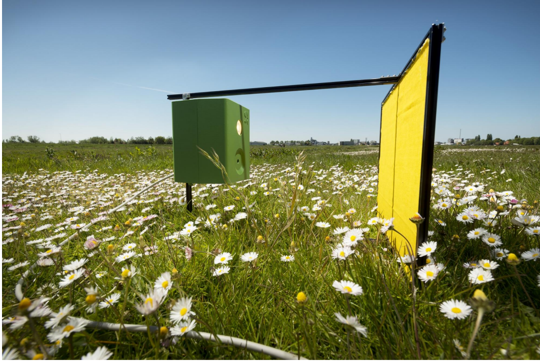
Figure 2.1: One of the cameras used to collect the data. The green box on the left contains the camera, lamp, SD card and the Raspberry Pi. Seen on the right is the yellow screen of which photos are taken every ten seconds.
